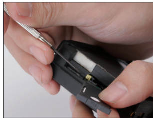
Removing the SIM holder.
